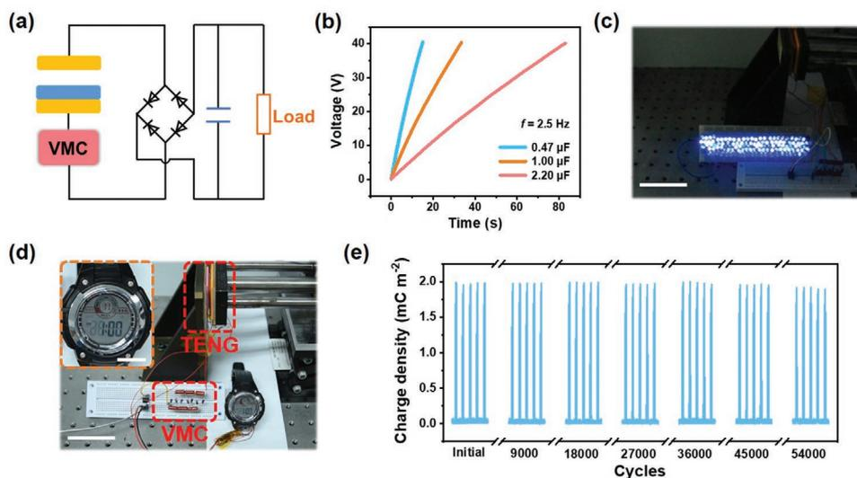
**Figure 4.** Demonstrations of the high equilibrium state TENG to drive devices. a) Circuit diagram of TENG with an energy storage unit for powering electronics. b) Charging curves of different capacitors at 2.5 Hz by two TENG devices in parallel. c) LEDs lighted up by high equilibrium state TENG (scale bar, 5 cm). d) A digital watch driven by high equilibrium state TENG (scale bar, 5 cm; scale bar of insert, 1 cm). e) Stability test of high equilibrium state TENG with 54 000 operation cycles.
