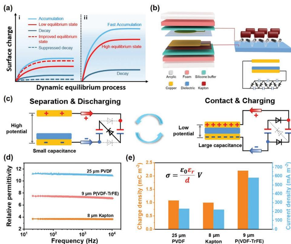
**Figure 1.** High equilibrium state and working mechanism. a) Schematic diagram of charge accumulation, charge decay, and dynamic equilibrium process. b) Structural illustration of self-charge excitation TENG in this work. c) Working mechanism of self-charge excitation TENG during periodic contact-separation process. d) Relative permittivity of three different dielectric layers. e) Surface charge density and output current density with three different dielectric layers.
