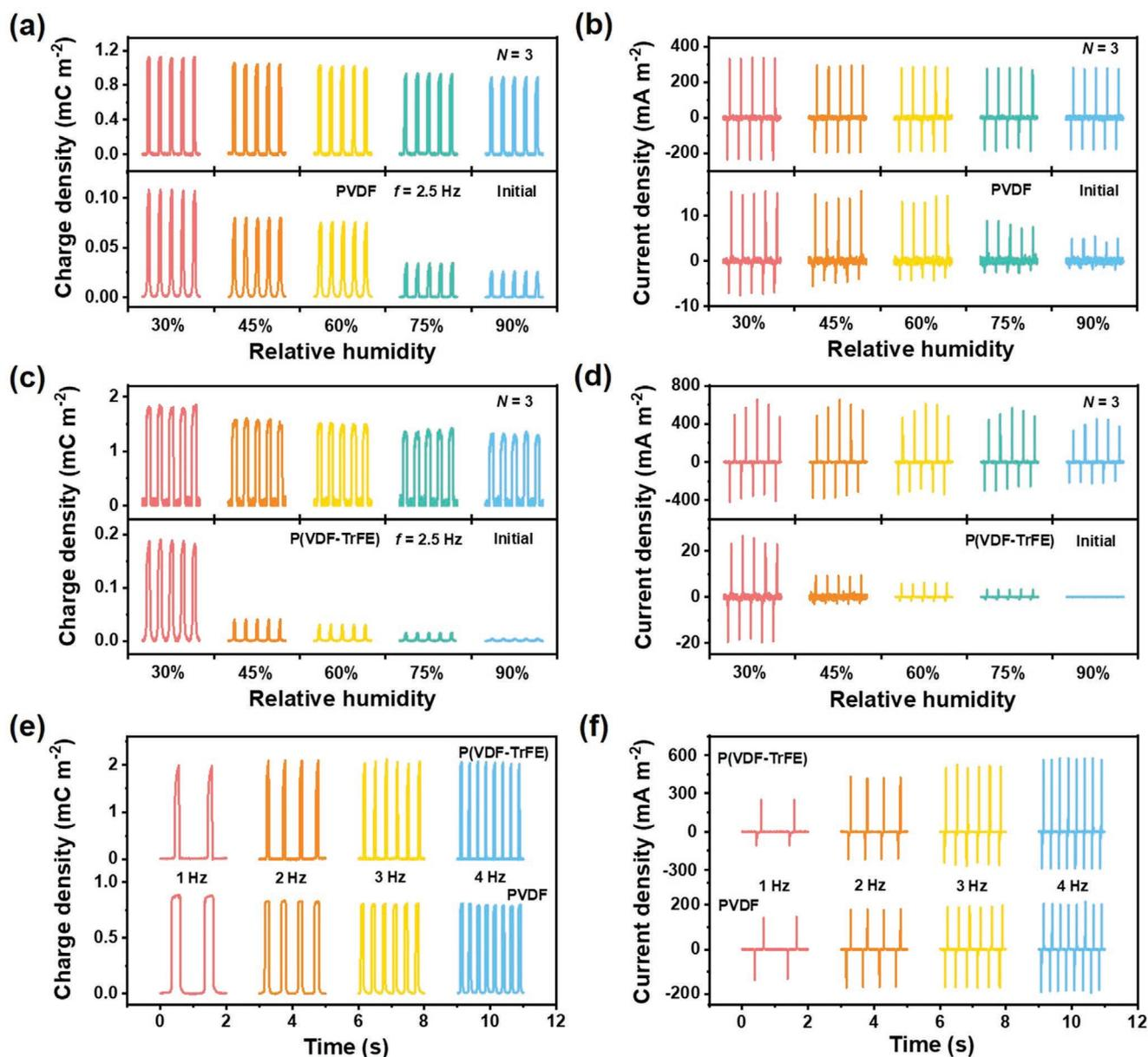
**Figure 3.** Equilibrium state under high ambient humidity. a) Charge density and b) current density of TENG with PVDF under initial state and  $N = 3$  when changing ambient humidity. c) Charge density and d) current density with P(VDF-TrFE) under initial state and  $N = 3$  when changing ambient humidity. e) Charge density and f) current density of TENG with PVDF and P(VDF-TrFE) under various operation frequency ( $N = 3$ ).
